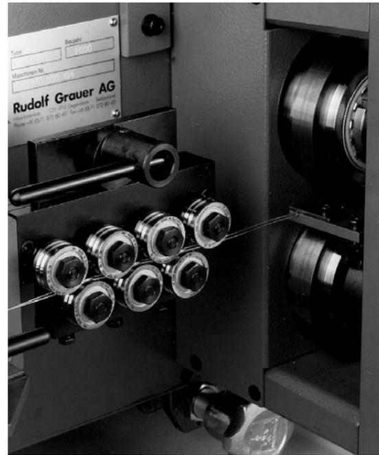
*The cutting unit can be simply shifted as a whole unit into any position within the full length range. Accurate cutter adjustment is carried out within a few seconds. Cutting heads are available for all normal shapes of cut and are interchangeable.*
