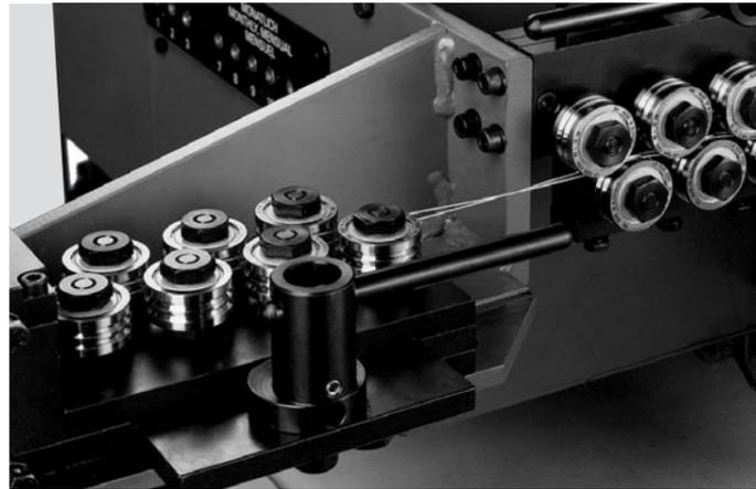
*Accurate guidance of each wire is fundamental to a perfect multi-wire process. A straightening system with 7 vertical and horizontal plane rollers, guarantees the necessary straightening quality for the whole range of wire diameters. Three rollers on each plane are individually adjustable and a quick-release hinge allows convenient handling.*
