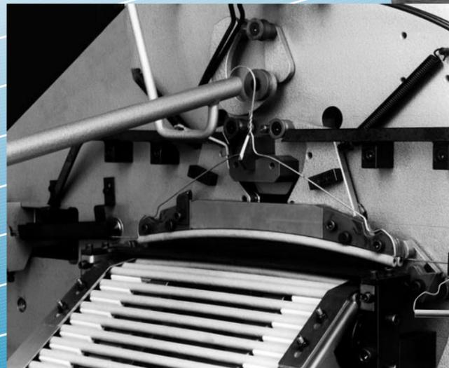
**2.** At forming of the shoulder, the two shanks of the hanger will be curved upwards through the bending rolls.
